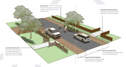
The FHWA recognizes this design as a potentially appropriate option for minor rural roads with low volumes (Average Daily Traffic or ADT<2000 vehicles/day) of traffic traveling at low speeds (<30mph) - see figure to the right.
